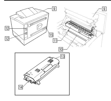
9 **Upper Unit:** Open to replace the Imaging Cartridge and to clear misfed sheets of paper.
